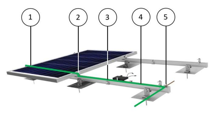
Items are listed in the fault current path in order from the PV Panel to the Grounding Lug:
